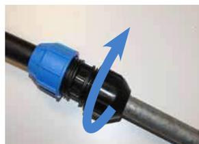
4. Hand tighten the nut and then tighten further with a proper standard tool. Do not screw the universal nut without pipe
